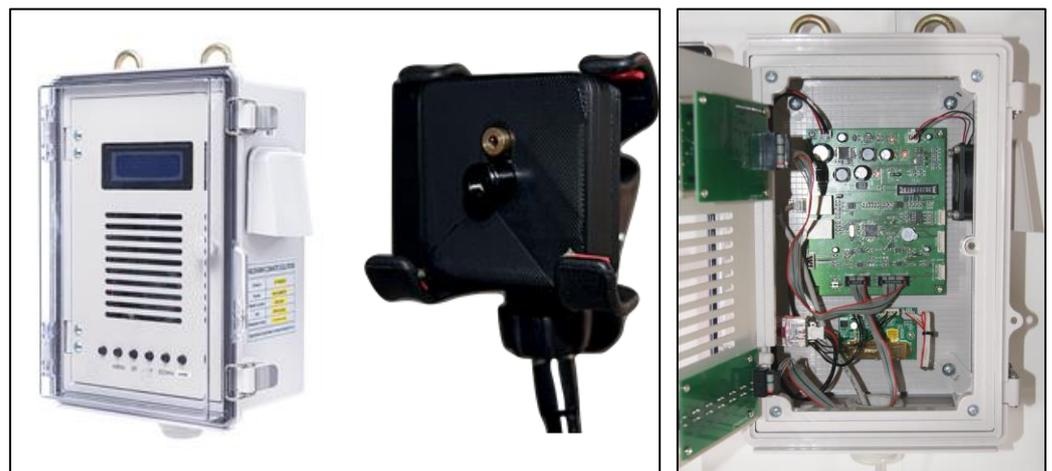
**Figure A1.** A prototype of new hardware for measuring leaf temperature. The hardware consisted of an information collection device and a non-contact infrared thermometer. RS485 MODBUS was used as the serial communication method, with a communication speed of up to 57,600 bps. A DC24V power supply was provided.
